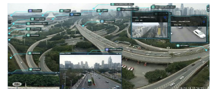
China TransInfo's Road Perception System—Low Point and High Point Traffic Accident Detection System
