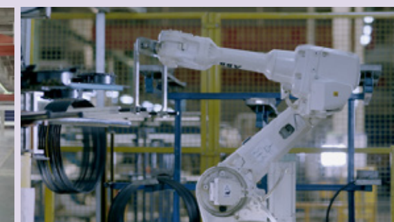
Automatic loop loading using steel wire winding intelligent robot
