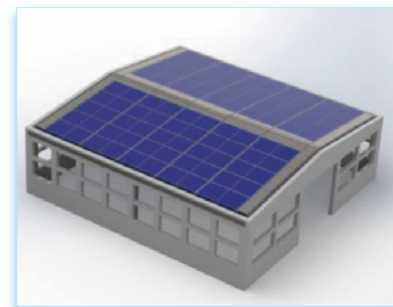
Dual Rooftop BIPV
