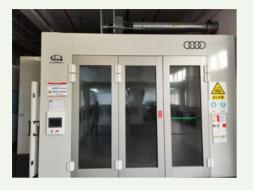
we have installed standard-compliant VOCs equipment for filtration and regularly replaces the equipment's filter elements. Our VOCs exhaust gas treatment process is suitable for medium-concentration pollutants, with workshop spray exhaust gases being drawn into the XHTML VOCs purification device by an air delivery system. The equipment consists of a primary filter, flat plate filter, and adsorption sections. Dry filtration is used to remove paint slag, with fine particles in the exhaust gas
