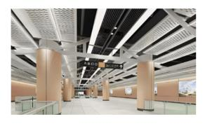
The panel lights used in the Xiamen Metro employ a design scheme featuring reflective plates and a sliding assembly structure. This design effectively reflects originally wasted diffuse light, significantly reducing internal light loss of the fixture, improving the light efficiency of the fixture. Consequently, it reduces the number of lamp beads and lowers the power consumption of the fixture, achieving reduced power consumption and increased efficiency in illumination.
