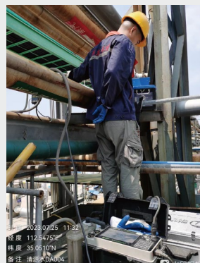
Monitoring of the Exhaust Outlet of the Raw Material Tank Area
