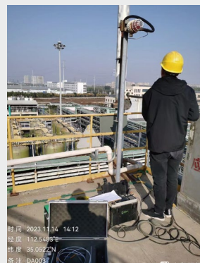
Monitoring of the Exhaust Outlet of the HEDP Unit
