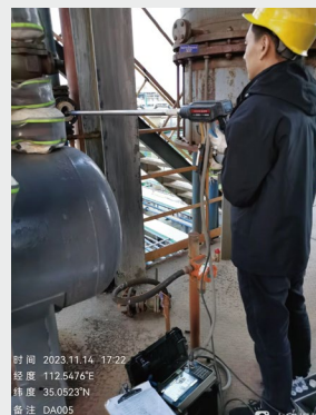
Monitoring of the Exhaust Outlet of the Hydrochloric Acid Unit
